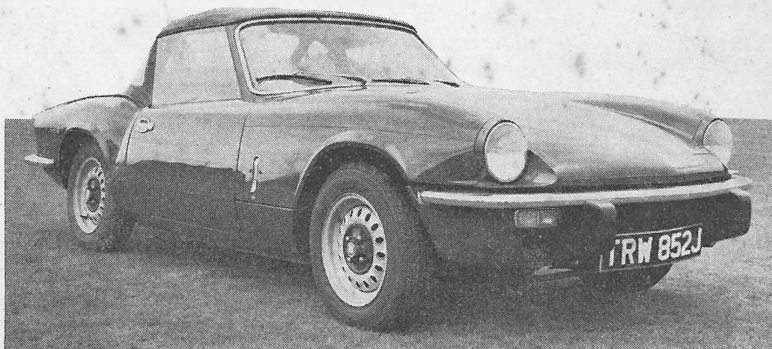
Spitfire Mk IV is restyled for the '70's: Rakish front with quasi-Stag rear; sporty pressed steel wheels new hood and door handles, deeper screen plus a completely revised rear suspension system
