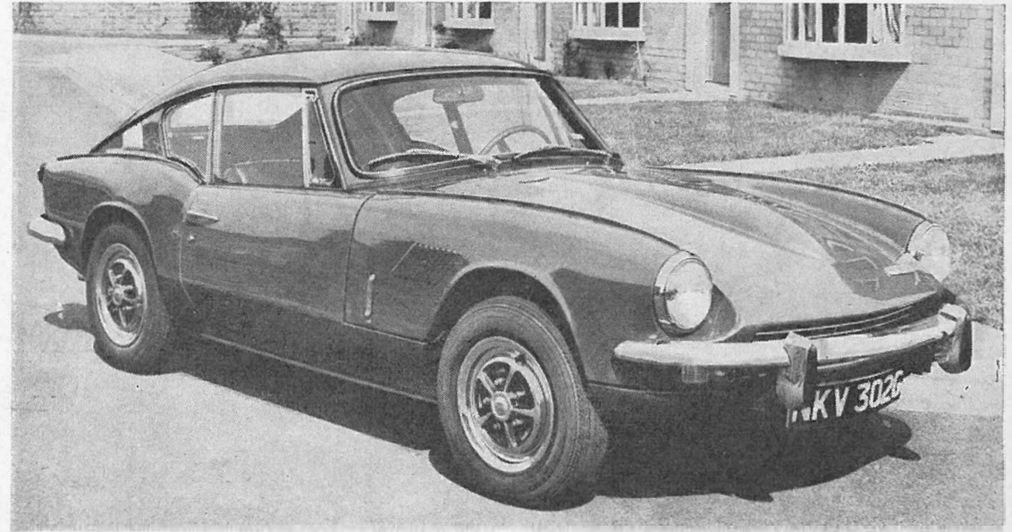
GT6 Mk 11 retains the same basic body shape of its predecessor but has louvred vents on bonnet and wings, raised front bumper, through-flow ventilation and sporty nave plates
