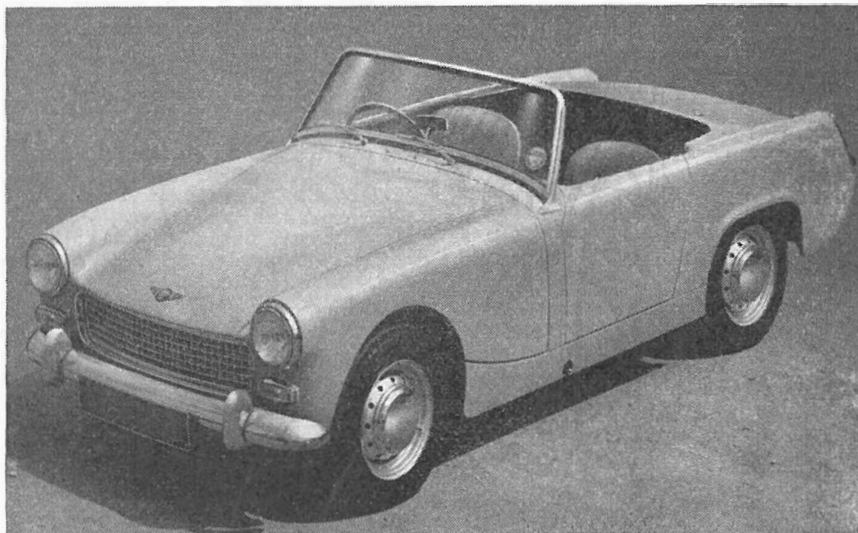
DISTINGUISHING FEATURES. Mark II versions of the model are easily recognized. New frontal treatment shows headlamps moulded into wings, and a full width radiator grille
