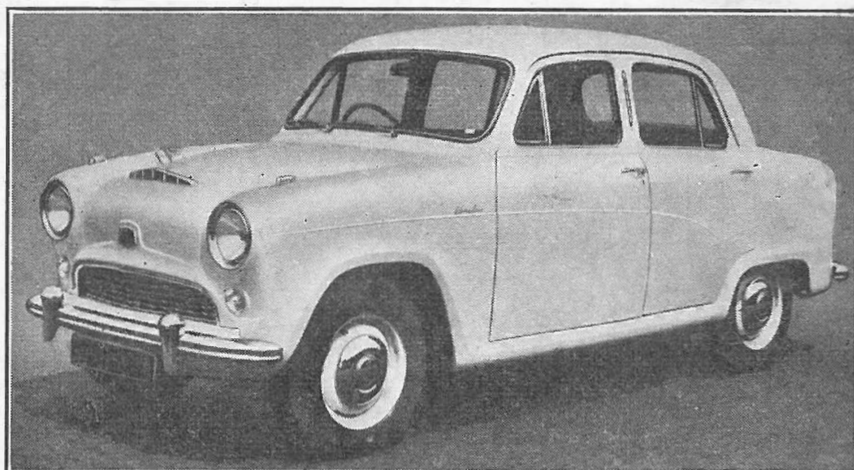
DISTINGUISHING FEATURES : Cambridge models marked a complete change of styling from the previous A40 models, with a wide grille, headlamps with a wide chrome bezel and a restyled boot
