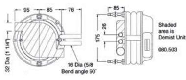
**080.500** With straight pipes and no demist facility 080.501 With straight pipes and demist facility 080.502 With bent pipes and no demist facility
