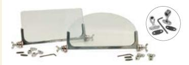
Choice of two made with Triplex laminated glass conforming to RAC competition regulations. Polished aluminium frame with chrome fittings. Width 406mm (16")
