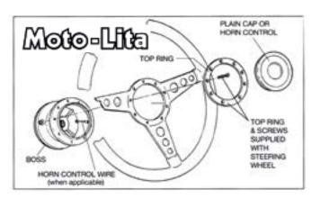
Mota-Lita bosses are machined from aluminium alloy castings and are stove enamelled wrinkle black. Each boss is splined to fit a particular steering column, and enables you to fit the Moto-Lita steering wheel of your choice. It is important to have the correct boss for your car. Please select a boss from the list below. If your car is not included here please phone our order line with details of your car: make, model and year
