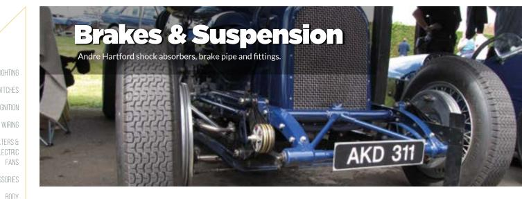
Andre Hartford Shock Absorbers are suitable for use on all makes of vintage car, and for all types of road and track events. This is the latest high efficiency model
