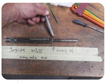
**Step 8.** The sliding shaft must be cut to length.
