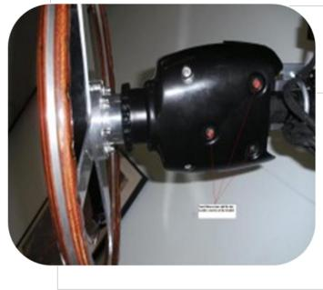
**Step 4.** Remove the housing from the steering column.
