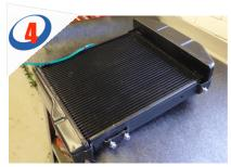
A. Working on a bench, ensure all six mounting bolts move freely.
