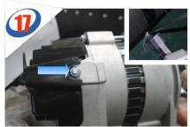
A. Ideally, the kit should be used in conjunction with an alternator conversion. B. Many alternators have a spare earthing point on their casing body - perfect for the EFC black earth lead.
