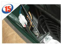
A. Now push the terminals into the connector block, ensuring their small lock tabs locate.
