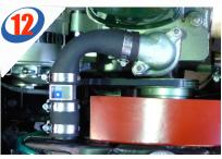
Fit the hose/EFC assembly. Do not fit the black EFC dust cover until final adjustments are made later. For fitment to the bottom hose, ensure the EFC adjusting slot is accessible.
