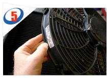
A. Position the fan so that the wiring will exit at the top of the radiator.
