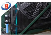
A. Undo the lower bolts and pivot the radiator back into position.
