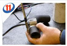
A. Fit both pieces of hose to the EFC ensuring the open top of the EFC points in the correct direction for access to the white slot when adjusting later. B. Fit both hose clips, ensuring they are accesible from above.
