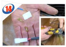
A. Now connect the wiring from the EFC/ relay to the fan connector block.
