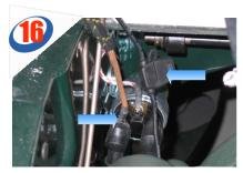
A. The inline fuse kit included (upper arrow) connects the main red feed from the EFC to the battery/loom terminal of the solenoid (lower arrow).
