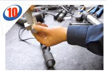
A. Measure the centre of the EFC as shown. It should be 25mm.
