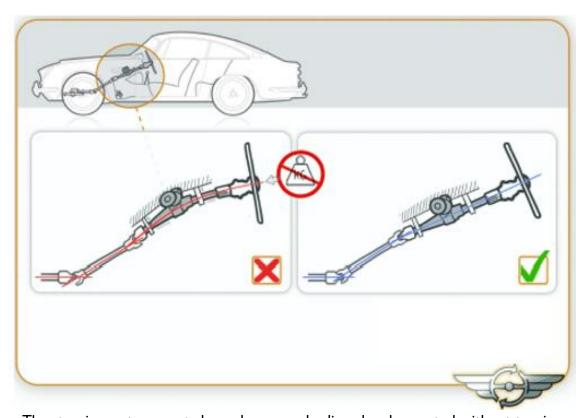
The steering system must always be properly aligned and mounted without tension.
